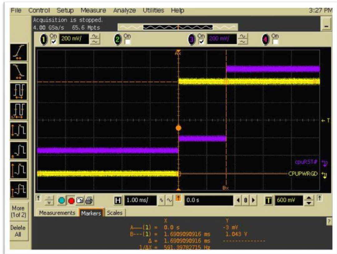
Figure 4. Example Snapshot of CPU Reset After the Power Good Assertion
