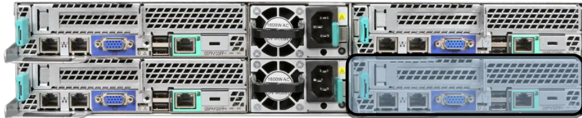
Compute Node 1 – Control Panel Node
