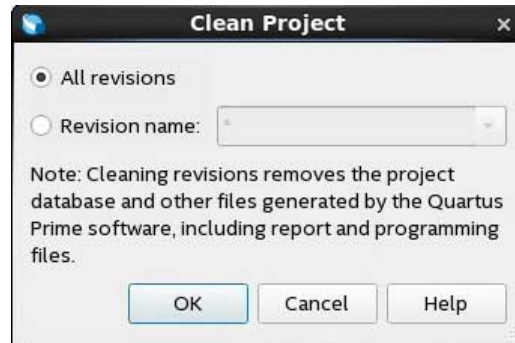
Figure 17. Clean Project Dialog Box Cleans the Project Database
