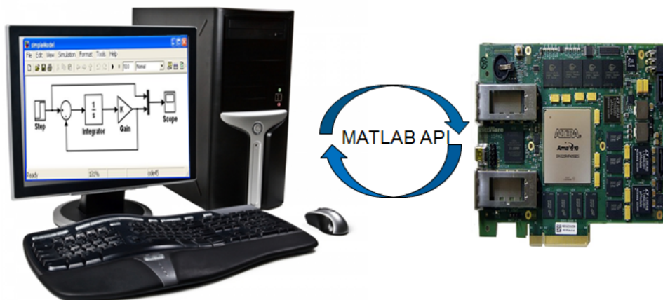
Figure 128. Hardware in the Loop Host-Target Setup
