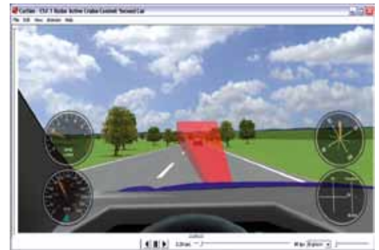
Figure 19: Simulation of Adaptive Cruise Control using CarSim.*
