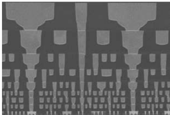
Figure 1: SEM image of interconnect stack up to MT8
