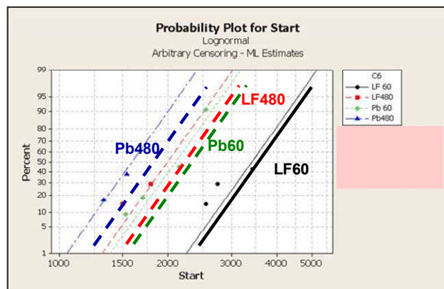
Figure 6: LF Temp cycle performance in long dwell time testing
