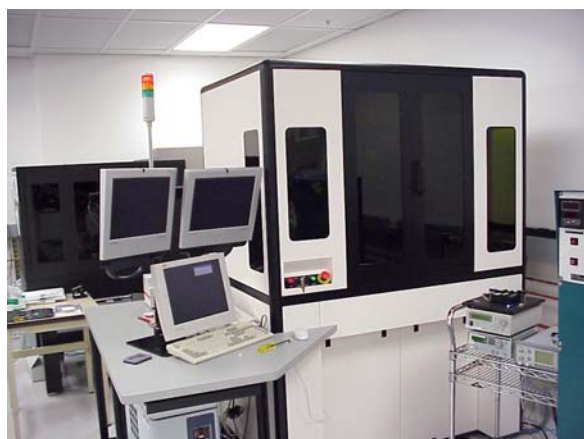
Figure 3: Automated welding system developed at Intel for high-throughput alignment processes
