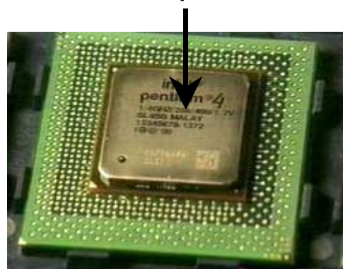
Figure 8(a): Use of IHS for Pentium® 4 processor
