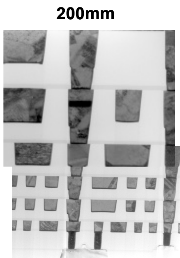
Figure 12: 200mm/300mm interconnect TEMs
