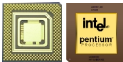
Figure 3: The Intel® Pentium® processor package in a ceramic PGA with a heat spreader
