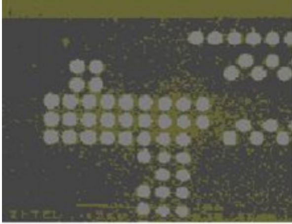
Figure 10: X-ray image of initial sample with prebake showing solder bumps
