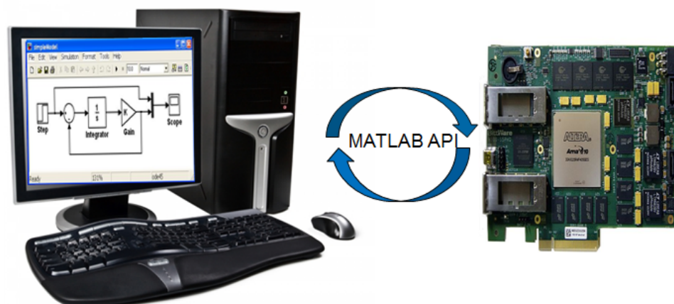
Figure 131. Hardware in the Loop Host-Target Setup
