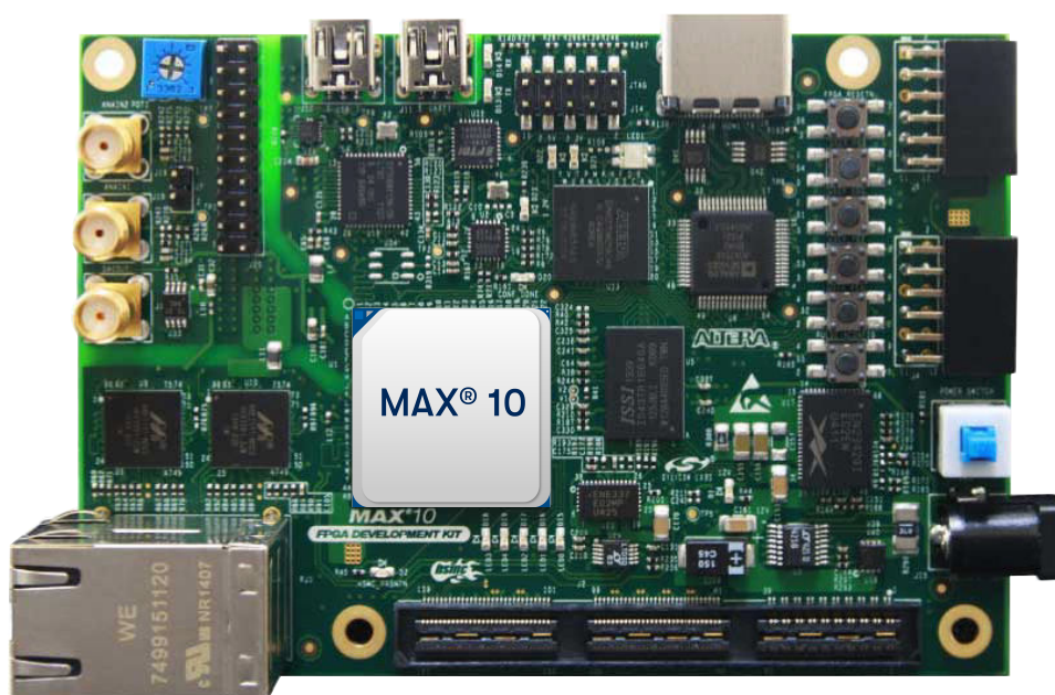
Figure 1. MAX 10 FPGA Development Kit—Top View
