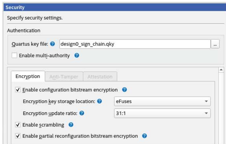
Figure 5. Partial Reconfiguration Bitstream Encryption Setting
