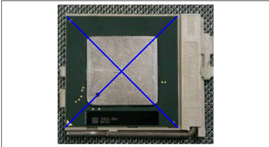
3. After the marks are scribed, clean the desired thermocouple attach location with a mild solvent and a lint-free wipe or cloth. Alcohol or acetone should suffice. Remember that the cleaner the part is, the stronger the bond will be after curing.
