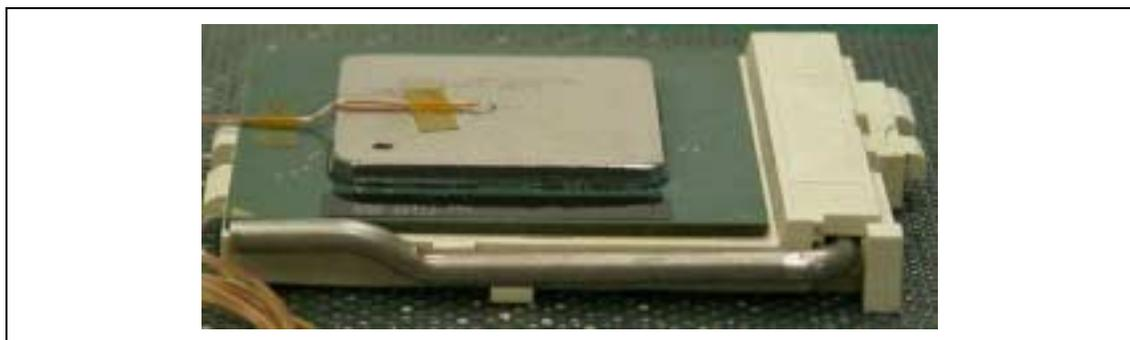
7. With the thermocouple in place, the epoxy can now be mixed and applied. Follow the manufacturer's directions for mixing the epoxy.
