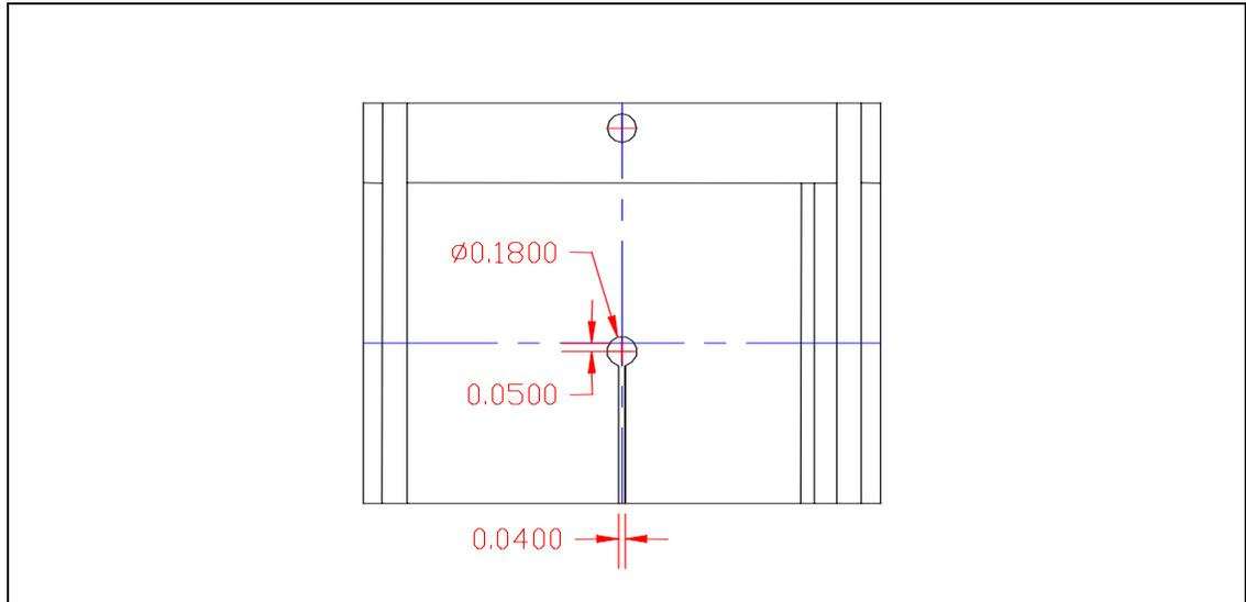
**Note:** Dimensions are in inches. Centerlines in drawing correspond to the thermocouple location (geometric center of IHS).
