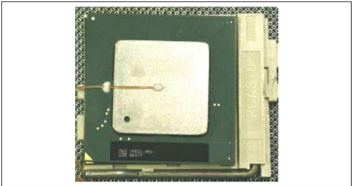
10. To cure the epoxy, put the part(s) in an oven set @ 150°F (65°C) for a period of 1 hour. Make sure the vibration in the oven is minimal to prevent the thermocouple bead from moving. Another alternative is to cure the epoxy at room temperature for at least 12 hours. (Some epoxy may have different cure times. Refer to the manufacturer's instructions.)
