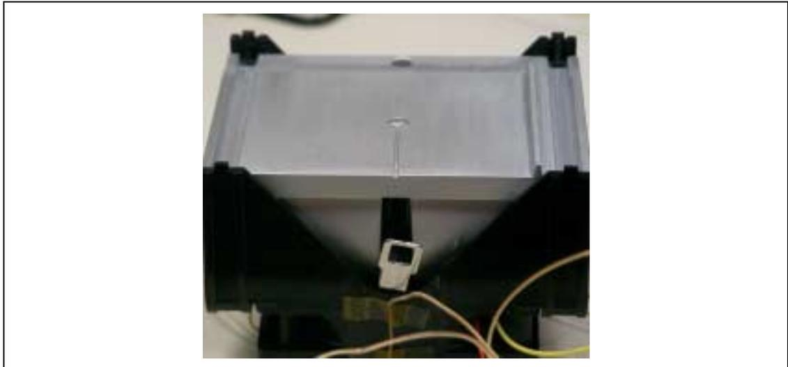
**Figure 7-8. Example of Dimensioning for Thermocouple Groove**
