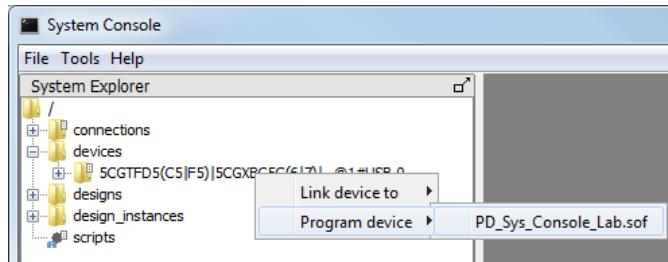
10. Expand the component in the **devices** section to see the components in the system that are connected to the Avalon bus in the **(hpath)** section or to the JTAG bus in the **(link)** section.
