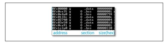
Using the linker, a new global variable is created in the RODATA section with the required size to hold the entire global variables metadata information:
