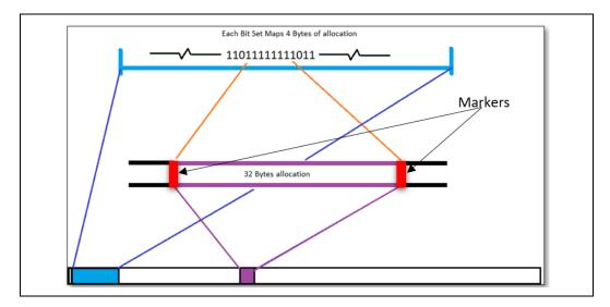
If a pointer to the heap points to mid-allocation (offset), we can calculate the location of the representation of the address in the bitmap and search for the beginning or end of the pointer and calculate the size of the allocation to be compared against the input we need to validate.
