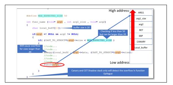
To solve this issue and get the size of "local\_buff" we leverage a feature of compilers that embed data that allows debuggers the ability to get function back tracing information. We use this same data to gain runtime knowledge of the function stack frame size.
