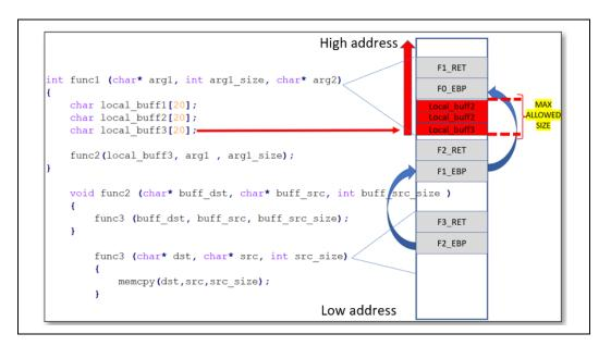
To make sure this structure on the stack will be generated a compiler option "-fno-omit-frame-pointer" MUST be used.
