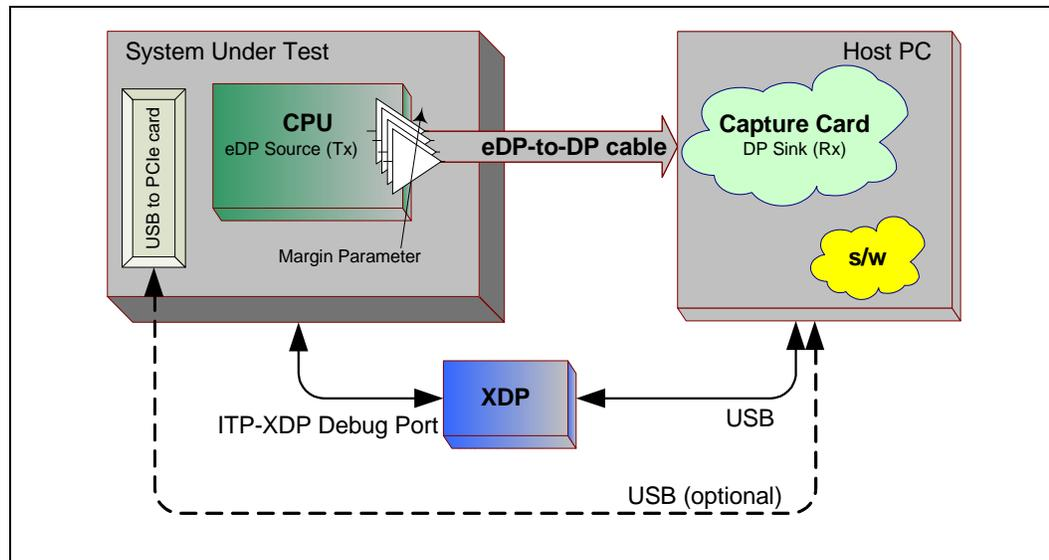
The margin parameter used for the eDP test is Tx amplitude swing. Nominal swing is defined as Step 0, the nominal margin position (see [Figure 3](#)). Going down with steps means lowering the swing. When a fail condition is met, the margin we seek is the distance of the current step from the nominal position. Going up with steps, i.e., raising the swing, is also possible though it would produce no fails because the receiver copes better with an amplified signal.
