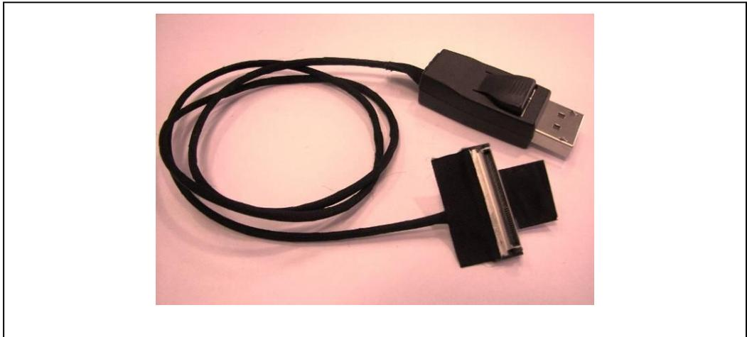
The typical cable's part number is LA10EM006-2N. Its length is 22" (559 mm). The cable length has to match 4 db insertion loss at 1.35 GHz. The frequency of 1.35 GHz is the first harmonic of the 2.7 Gb/sec DisplayPort data signal. The data lanes' wires are twin-ax coaxial cables.
