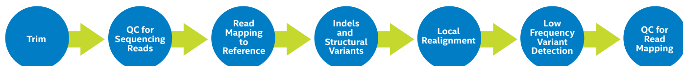
Figure 3: Standard Qiagen WGS Variant Calling Workflow.
