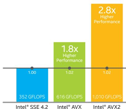
**Figure 1.** Measuring performance on the same processor using Linpack\* benchmarks shows substantial increases from Intel® Streaming SIMD Extensions 4.2 (Intel® SSE 4.2) to Intel® Advanced Vector Extensions (Intel® AVX) and from Intel AVX to Intel® AVX2, with up to 2.8x the GFLOPS throughput when comparing Intel SSE 4.2 to Intel AVX2.<sup>2</sup>
