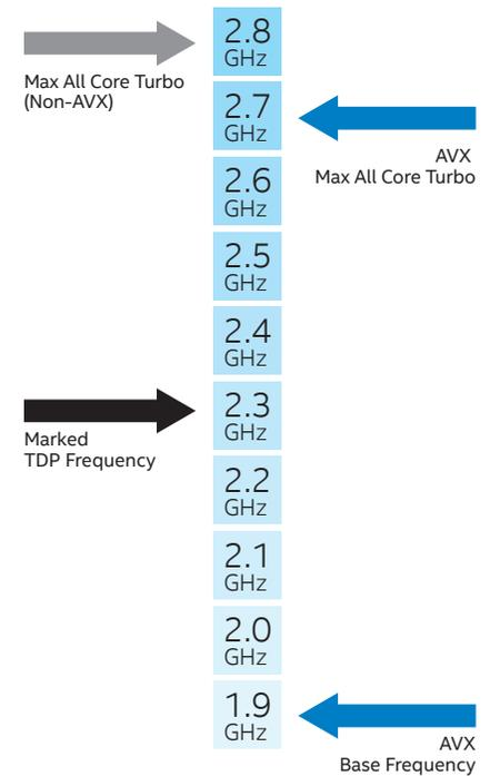
**Figure 2.** The new Intel® Advanced Vector Extensions (Intel® AVX) instructions could operate at or below the marked TDP frequency, while still providing up to two times the floating-point throughput.
