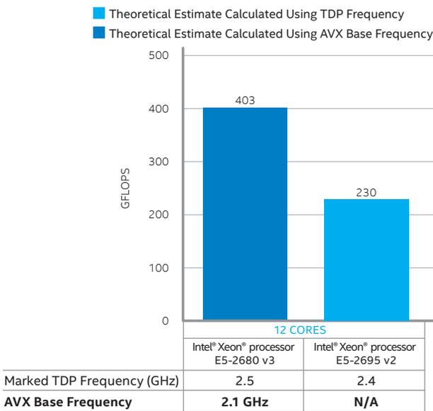
**Figure 3.** Calculating the theoretical peak FLOPS using the AVX base frequency results in up to a 1.7x increase in peak GFLOPS on Intel® Xeon® processors using Intel AVX2 over the value calculated using the TDP frequency on a previous generation processor with the same core count and similar frequency using Intel AVX.<sup>7</sup>
