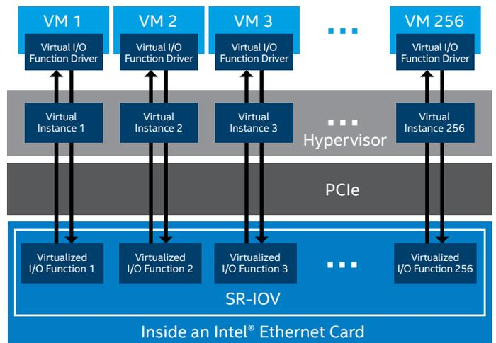
**Figure 1.** SR-IOV provides a way for the hardware capabilities of a PCI Express device (a network adapter in this case) to be presented to the operating system or hypervisor as multiple virtualized NICs without some of the hypervisor's overhead and processing latency.
