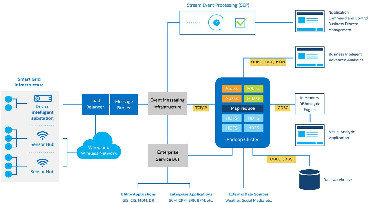
Figure 3: Proposed hybrid architecture for an energy data superstore
