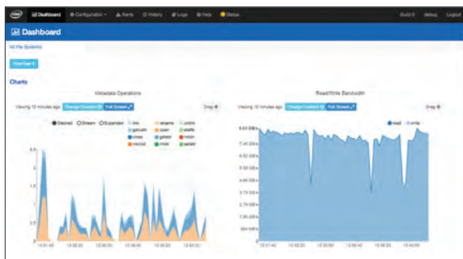
Figure 17. MCP read bandwidth at source with 20 data movers - large files. In our tests, MCP achieved 8.5 GB/s of read bandwidth while transferring one hundred 50-GB files at the source file system with 20 data movers.
