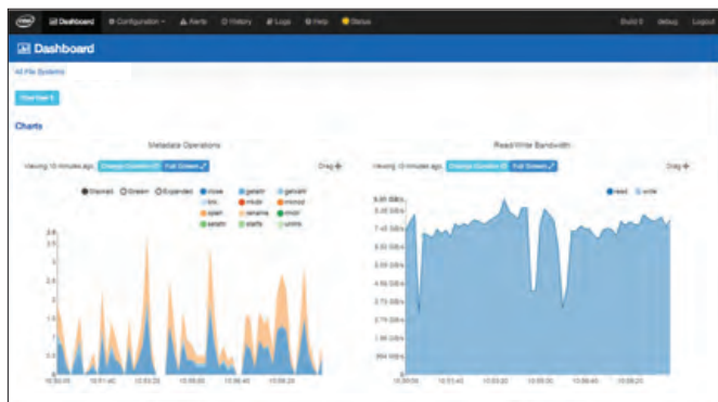
Figure 15. MCP read bandwidth at source with 8 data movers - large files. In our tests, MCP achieved 8 GB/s of read bandwidth while transferring one hundred 50-GB files at the source file system with 8 data movers.
