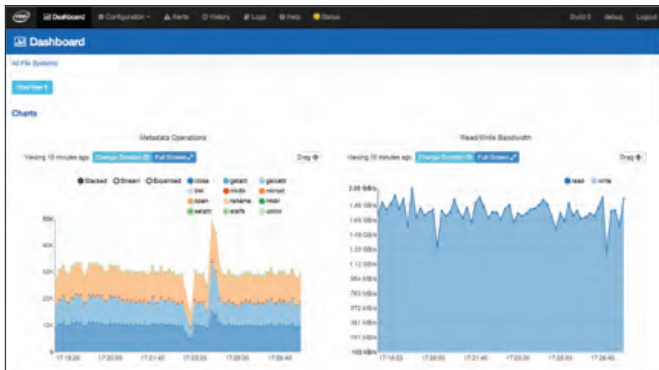
Figure 11. MCP read bandwidth at source with 8 data movers - small files. In our tests, MCP achieved 2 GB/s of read bandwidth and 30,000 sustained metadata ops while transferring 100,000 16-MB files on the source file system with 8 data movers.
