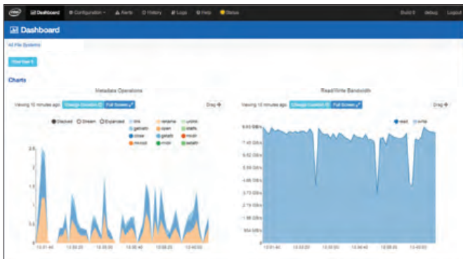
Figure 9. Fpart read bandwidth at source file system with 20 data movers - large files. In our tests, fpart achieved 8.5 GB/s of read bandwidth while transferring one hundred 50-GB files at the source file system with 20 data movers.
