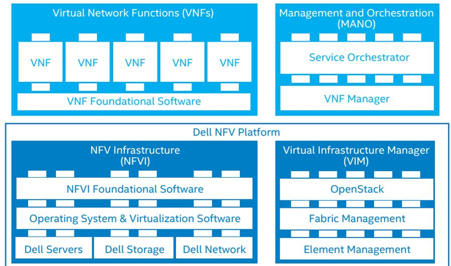
**Figure 1.** Components of the Dell NFV Platform.
