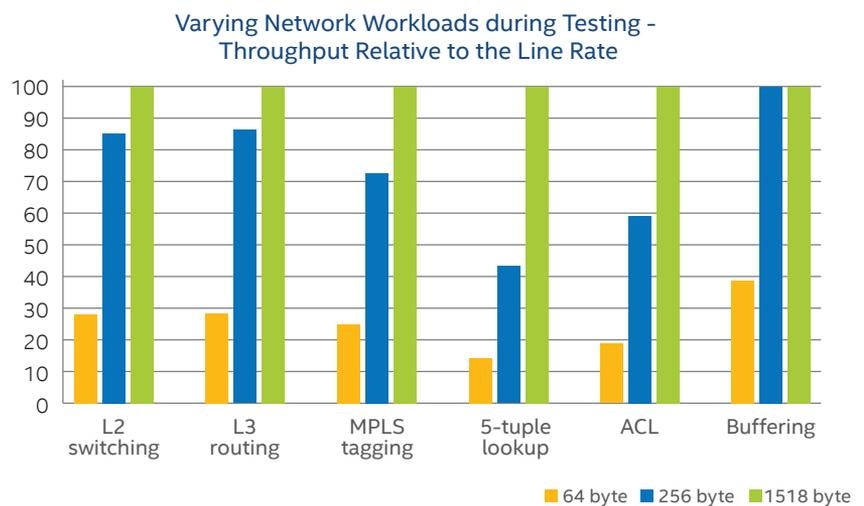
Figure 4. Test results for different network workloads.
