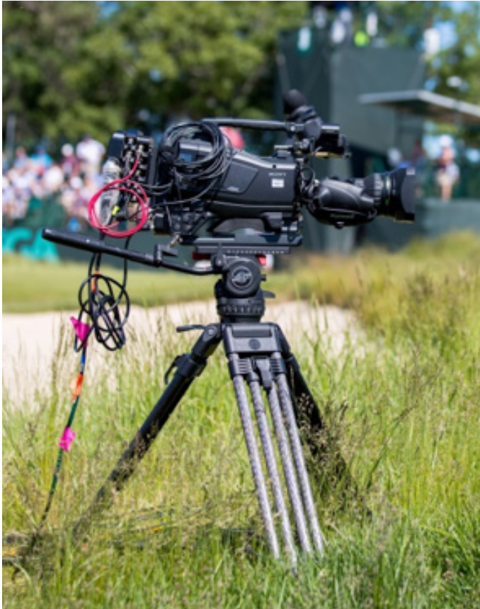
Figure 1. A remote 4K video camera connected to the Fox Sports network over a 5G link using spectrum provided by AT&T. Ericsson's 28GHz radio and antenna are located at the tower seen in the distance.
