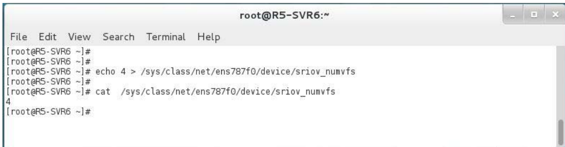
Figure 4. VF Creation via SysFS
