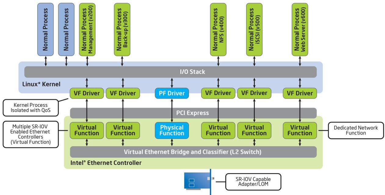
**Figure 4.** Port Partitioning implemented in a bare-metal Linux\* environment
