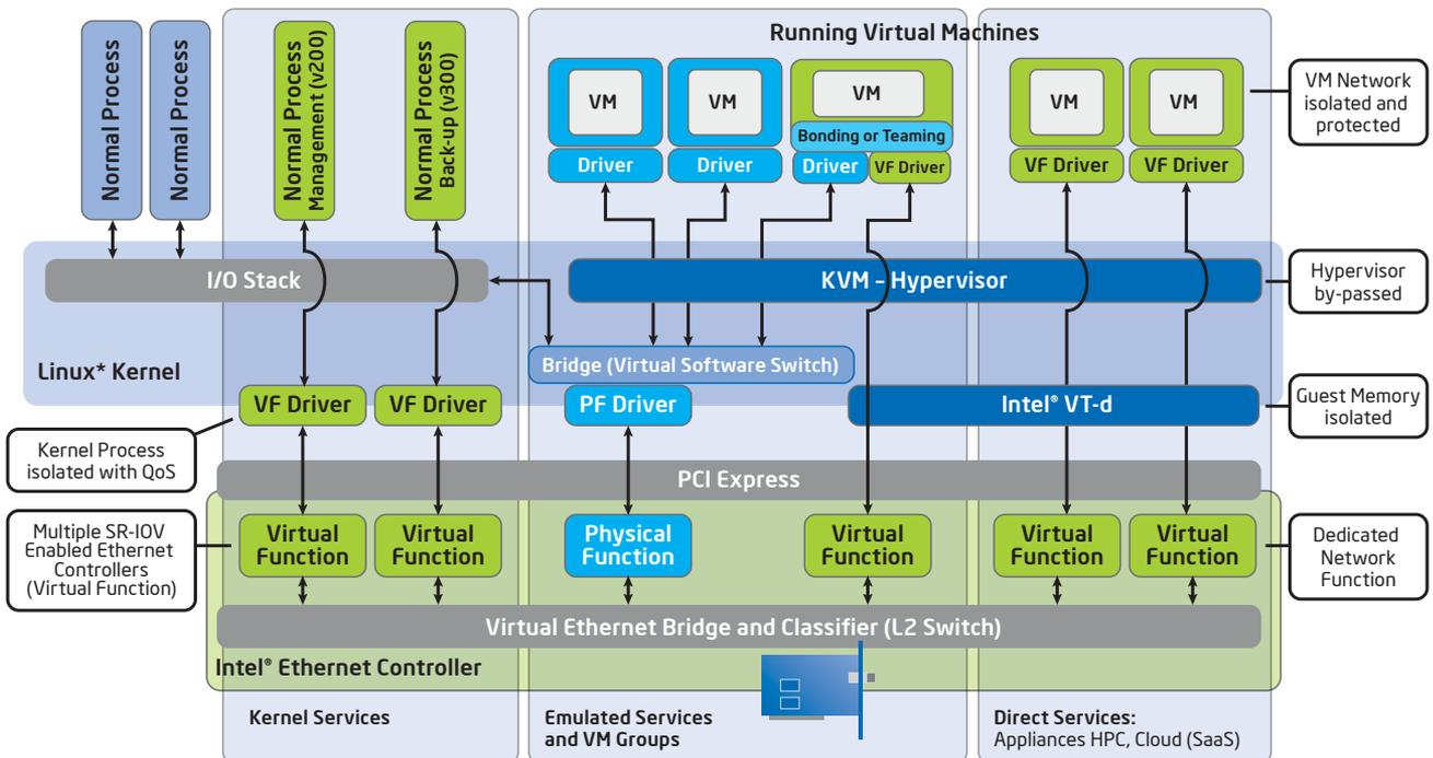
**Figure 5.** Port Partitioning in a combined bare-metal Linux\* and virtualized environment
