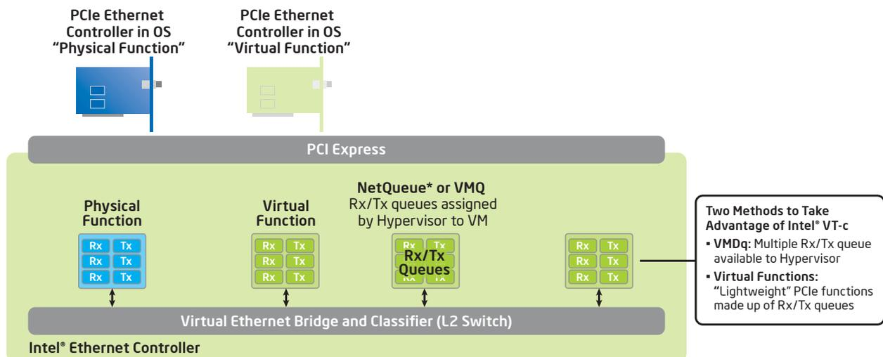
Figure 1. Overview of Intel® Virtualization Technology for Connectivity
