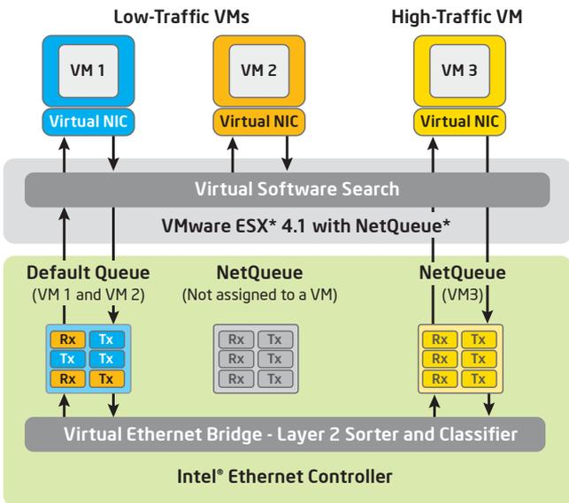
Figure 2. Virtual Machine Device Queues
