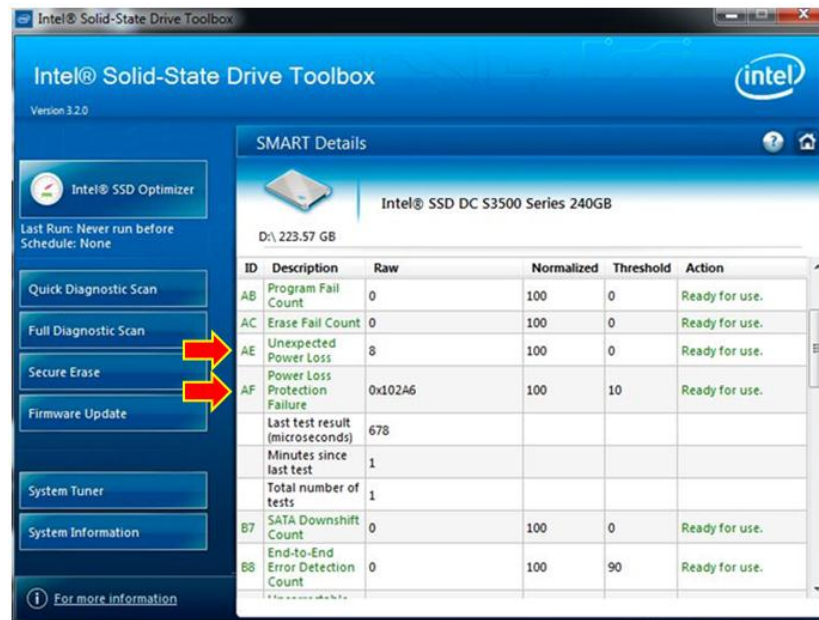
Figure 5: Intel® SSD Toolbox Reporting Sample PLI SMART Attributes on the Intel® SSD DC S3500 Series
