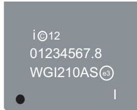
Figure 1-4 I210 Production Top Marking Example (Industrial Temperature Fiber)
