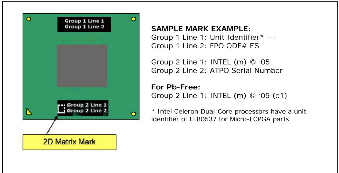
Figure 2. Intel Celeron Dual-Core Processor (Micro-FCPGA/FCBGA) Production Markings
