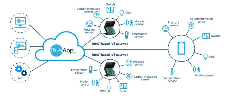
BlueApp.io supports various hardware adapters such as BluTerm\*, a set of Bluetooth adapters that read and convert RS232, RS485, BACnet\*, Modbus\*, 40 to 20mA, and 0 to 10V registers and sends the data to a Bluetooth Wi-Fi gateway and then to the cloud.
