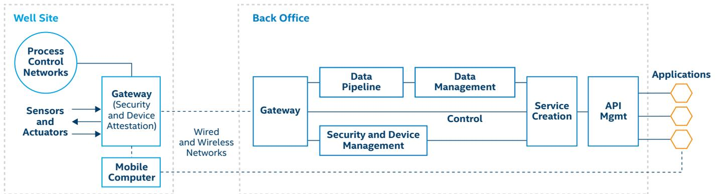
Figure 3. Conceptual architecture for upstream oil and gas
