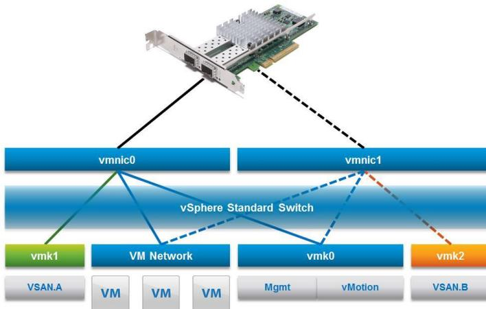
One vSwitch is used to connect both 10 Gb vmnics as uplinks. Four port groups, three of which are VM Kernel Adapters (or VMKs) are used to carry the varying traffic. Different VLANs are also used to segment traffic to the respective port groups and VMKs. Utilizing two 10 Gb links to carry all traffic greatly simplifies the network requirements by reducing the number of network adapters, network cables, and switch ports required.
