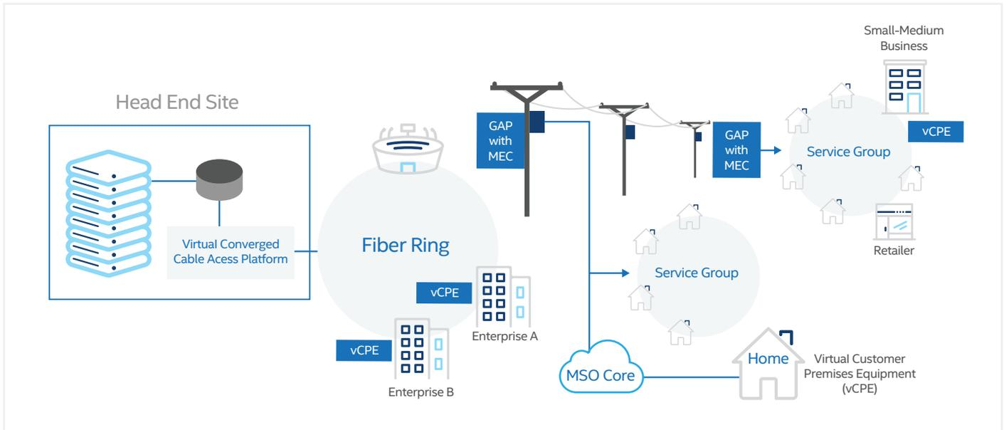
Figure 4. MEC in GAP Is Located Close to Subscribers
