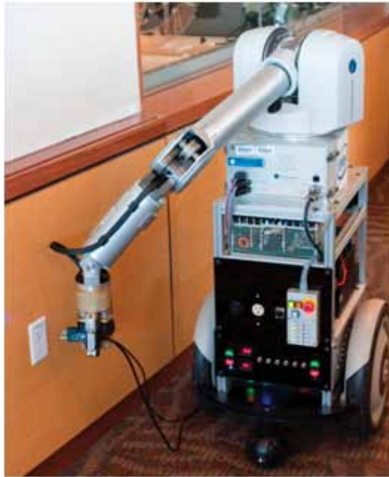
Figure 3: Robot Marvin Uses Electric Field Pretouch both for Manipulation and for Sensing the Location of Electrical Outlets Source: Intel Corporation, 2010
