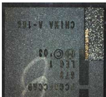
Figure 24: Mold compound removed only at upper right side
