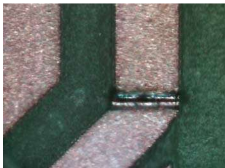
Figure 26: Trace width is approximately 28-microns wide
