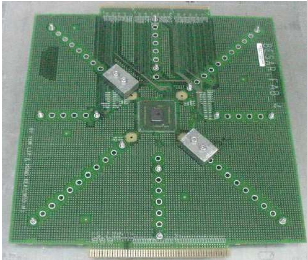
Figure 10: Shock test board used to test the component capability
