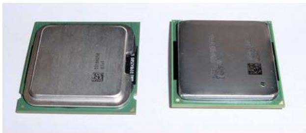
Figure 3: LGA775 and mPGA478 packages
