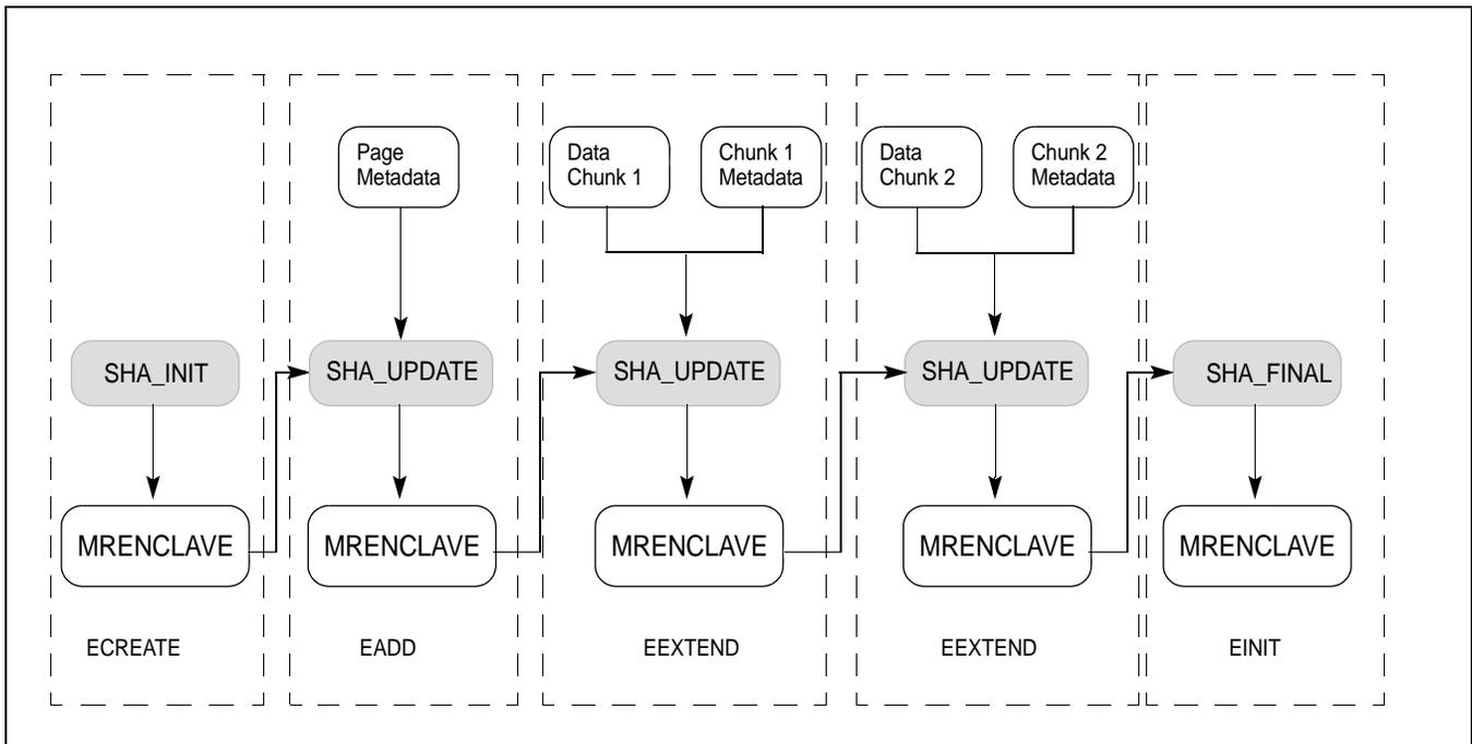
Figure 39-2. Measurement Flow of Enclave Build Process
