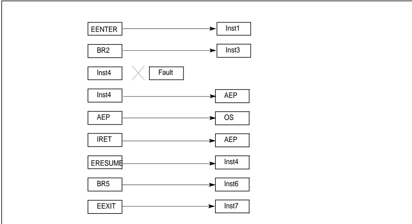
Figure 43-3. LBR Stack Interaction with Opt-in Entry
