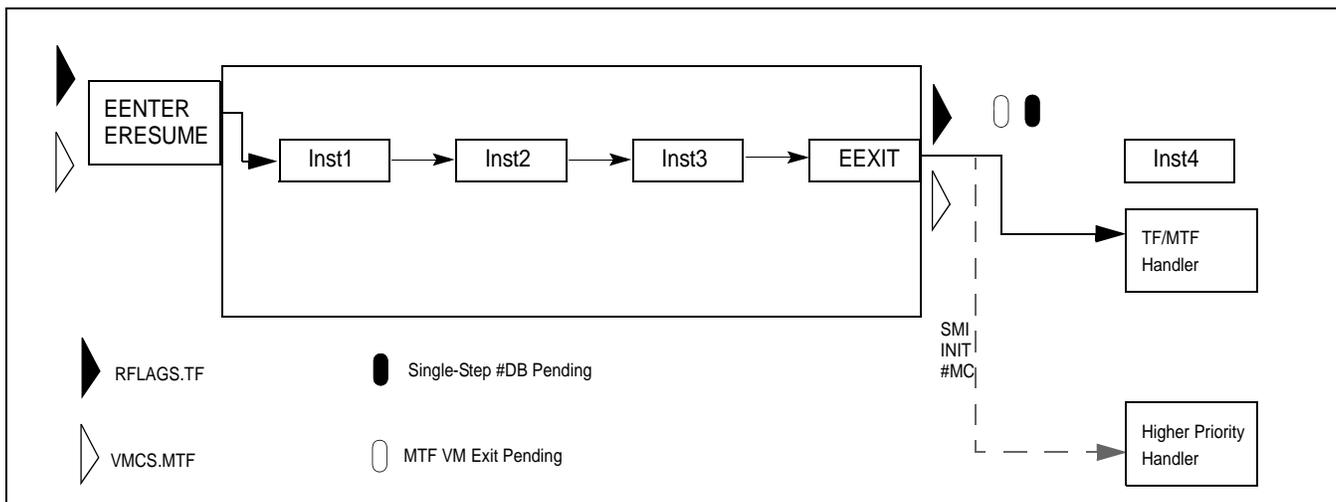
Figure 43-1. Single Stepping with Opt-out Entry - No AEX
