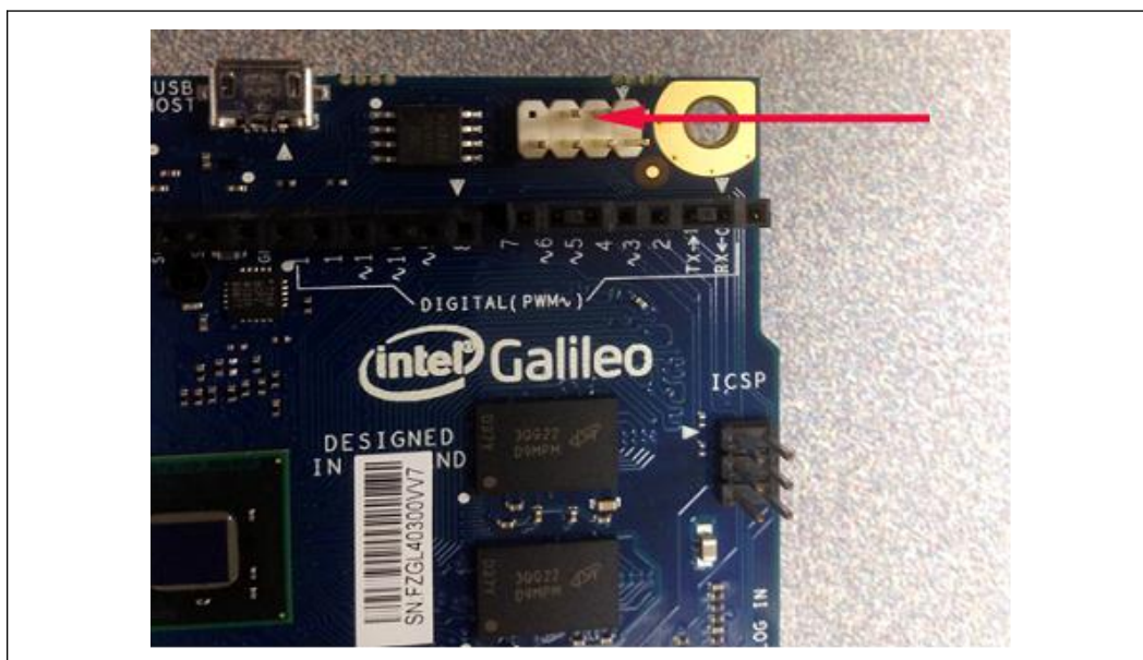
Figure 61. DediProg Header on the Target Device
