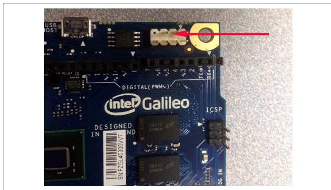
Figure 55. DediProg Header on the Target Device
