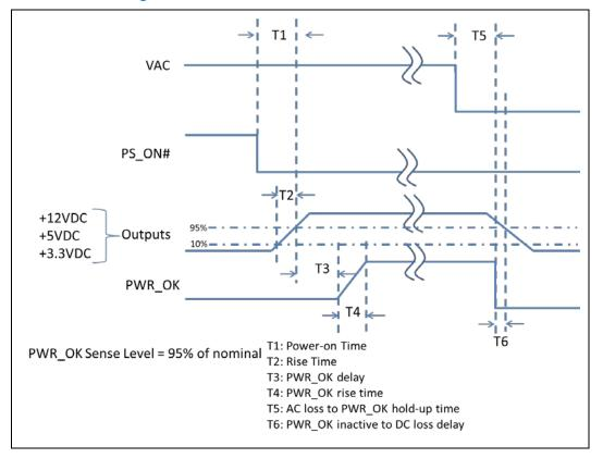
Figure 3-3: Power on Timing
