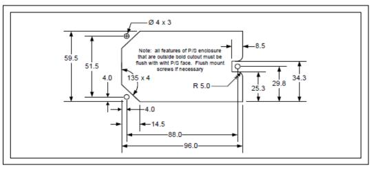
Figure 13-5: Recessed Fan Mounting
