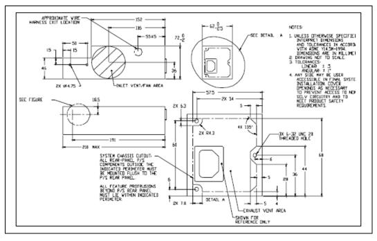
Figure 11-3: PSU Slot Feature Detail
