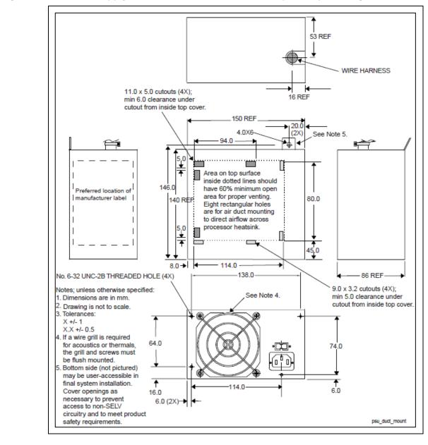
Figure 12-2: Power Supply Dimensions for Chassis that Require Top Venting
