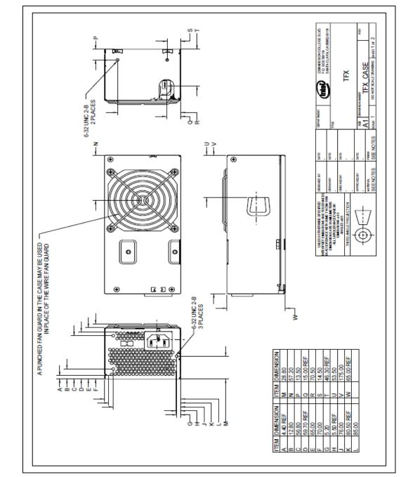
Figure 14-2: Dimensions and Recommended Feature Placements (not to scale)
