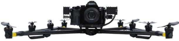
**First flight:** a single automated circle-of-interest flight around the cathedral at 100 meter altitude. Camera angle set to 45 degrees. Flight time around 14 minutes, with 169 images captured.
