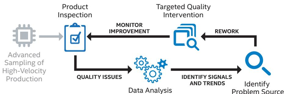
Figure 3. Quality rules are applied to real-time process data to determine whether material is viable to continue production, whether it requires rework, or whether it should be scrapped. Rapid responses to problems also increase uptime, accelerate output, and save money.
