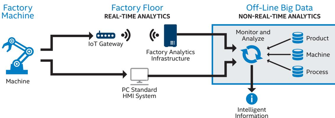
Figure 1. Data from edge computing and Internet of Things (IoT) is extracted for real-time analysis on the factory floor as well as big data analysis in off-line databases. Engineers have relevant statistical data at their fingertips at all times.
