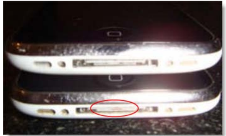
Figure 1: Built-in water damage sensors changed color if your phone has been damaged. But, they can be very hard to see.
