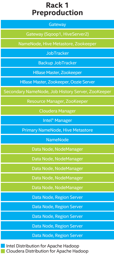
Figure 3. The preproduction environment enabled us to validate our processes. This environment was powered by 128 cores (using Intel® Xeon® processors) and eight data nodes populated with actual data volumes.
