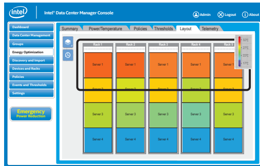
Figure 6. This detailed view of server locations within racks reveals that the servers in the top row are hot, a common occurrence that cannot be detected without server-level thermal monitoring.
