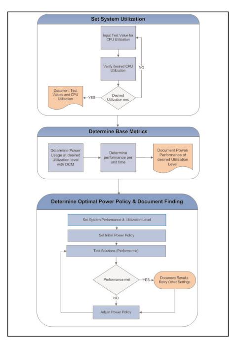
Figure 5. Detailed PoC and test methodology
