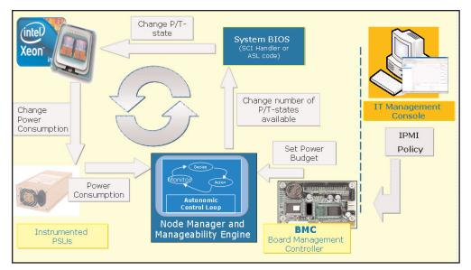
Figure 1. System and platform architecture for Intel Intelligent Power Node Manager and Intel DCM
