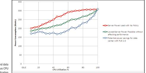
Figure 8. Projected CPU and data center power savings versus CPU utilization
