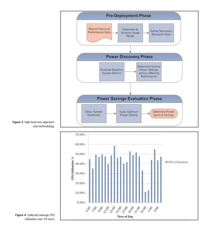
The team used the processes outlined in Figure 3 and 5 to determine the optimum power policy setting that matched the performance requirements of the historical performance of the servers. Using this systematic process made it possible to arrive at optimal power settings without impacting the system performance.
