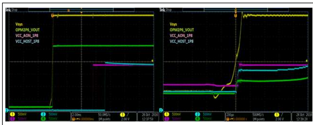
Figure 1. Intel® Quark™ SE Microcontroller C1000 Power Sequencing
