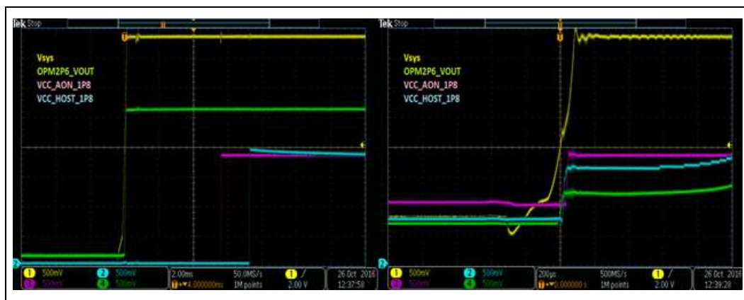
Figure 1. Intel® Quark™ SE Microcontroller C1000 Power Sequencing
