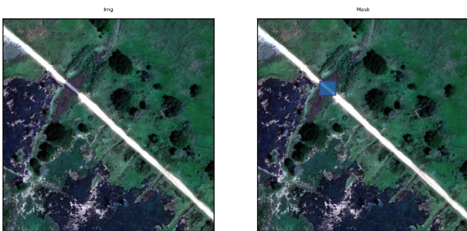
Figure 5. Generation of a bounding box around a bridge.
