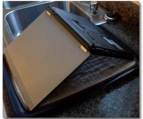
Figure 4: The key to saving your laptop after a spill is to drain it of as much moisture as possible. This will mean a lot of waiting for natural evaporation to take its course.
