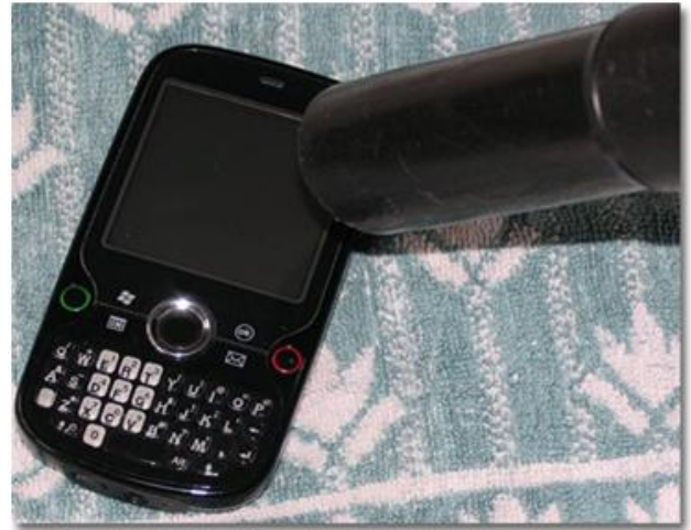
Figure 2: A vacuum cleaner can draw moisture away out of your phone, but only from a distance - too close, and the resulting static will do more harm than good.
