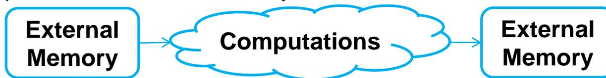
Unnecessarily going to external memory in the middle of computations, or reading input data multiple times, is a sure way to limit your kernel's performance.
