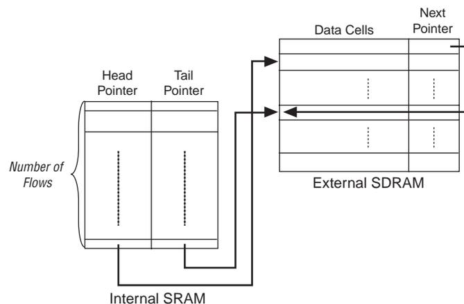
The Stratix GX M-RAM blocks are optimal for storing pointers to external memory locations. For example, with a 128-Mb SDRAM containing fixed 64-byte cells, Stratix GX M-RAM blocks can store both head and tail pointers for 64K flows.
