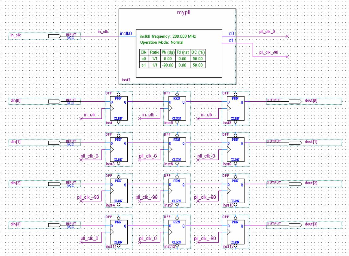
The PLL phase shifting technique will help improve  $t_{CO}$  but will not affect the  $t_{PD}$  as there is no clock network in the  $t_{PD}$  path. One approach to help improve the  $t_{PD}$  is to move the combinational logic close to the output pin to help reduce the routing delays.
